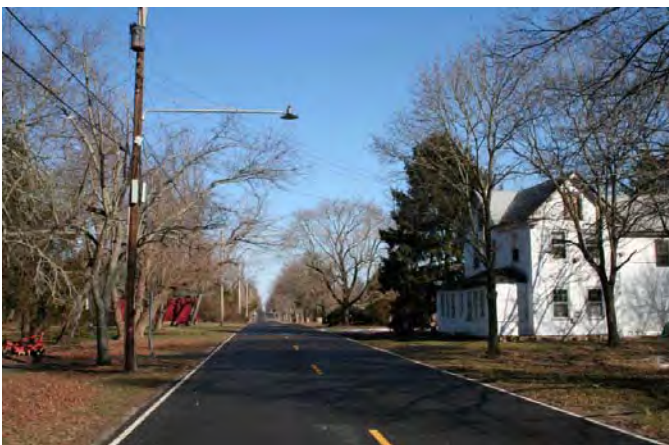
Caption: A modern “historic-look” rural light fixture (complete with electric eye) reflects the historic character, scale and simplicity of historic rural street lights in this agricultural district in New Jersey. Paul Daniel Marriott
